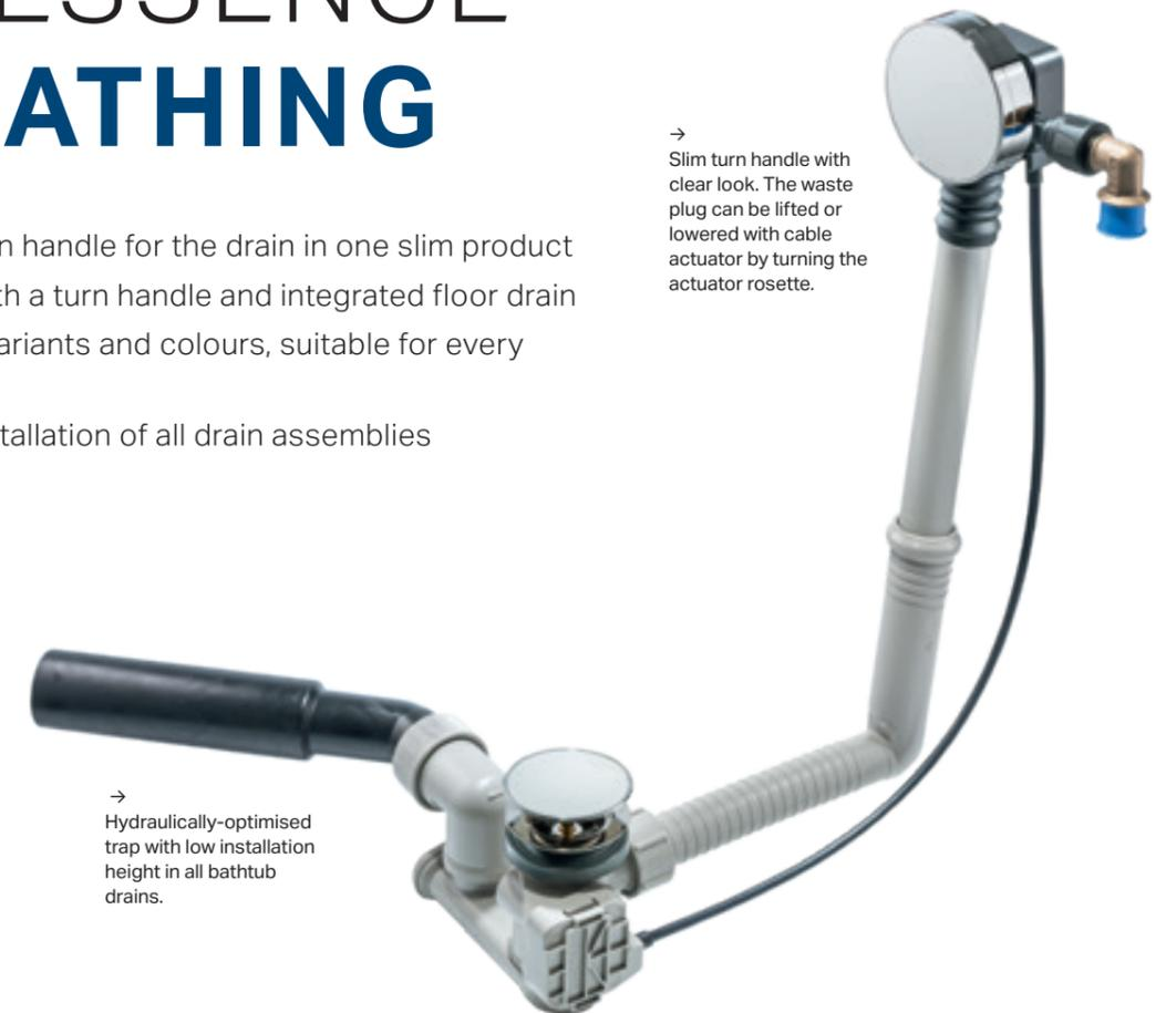
→ Slim turn handle with clear look. The waste plug can be lifted or lowered with cable actuator by turning the actuator rosette.
