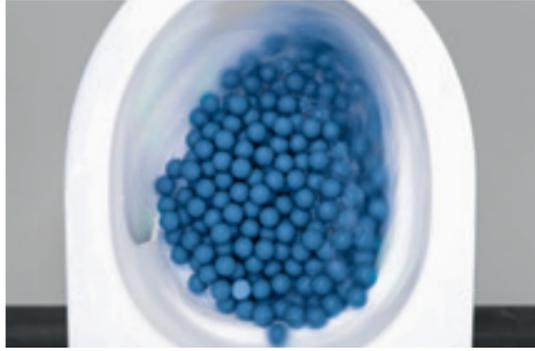
Flush performance is up to 10 times better than required by standard testing (DIN EN 997-2018).
